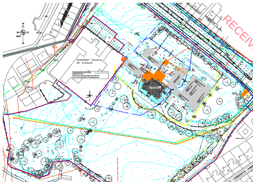
Figure 4 - Demolitions and diversion of services
